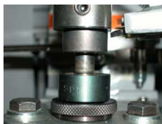
14. Remove the grommet. Stop the flywheel when the top die reach the bottom dead center.
