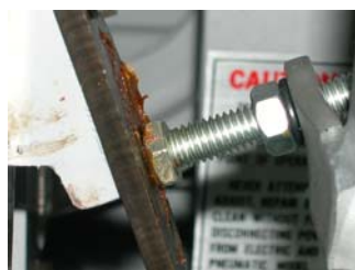
18. If the track come back too early, the track may hit the top die. Adjust this bolt for right timing.
