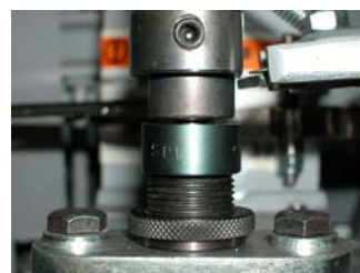
15. Use the ring nut to adjust the bottom die until you have proper gap between the top and bottom dies.
