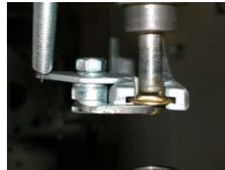
7. Check if the pin of the top die is in the middle of the opening at the end of the track.
