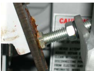
13. If the track is pushed away too early, the grommet may fall from the pin. Adjust this bolt for right timing.
