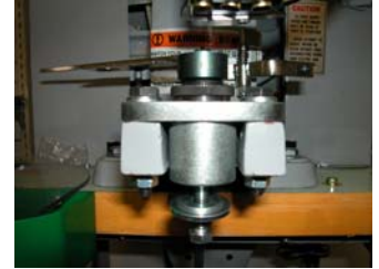
4. Replace the bottom die. Adjust the ring nut to keep the die low. Do not tighten the locking bolt at this time.
