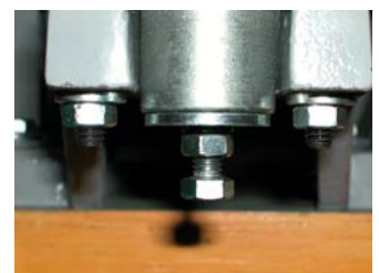
20. If everything looks O.K., tighten the nut on the locking bolt and re-install the safety guard and small table.
