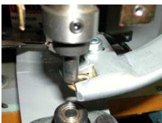
17. Turn the flywheel clockwise. The track should return without contacting the die.
