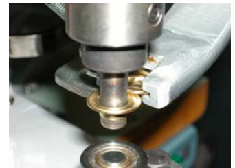
12. The pin of the top die grab the grommet from the track as the track being pushed away.
