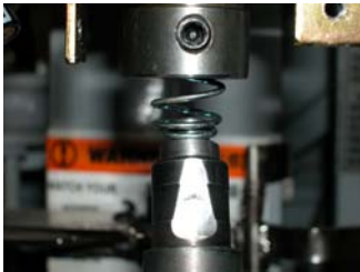
5. Replace the top die. Note the notch should face the set screw and the spring should be riding on the
