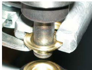
10. The shaft start to move down and the pin of the top die will go through the hole of the grommet.
