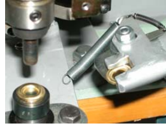
3. Remove the spring that pull the track from the hook.
