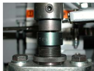
19. Repeat steps 8-18. This time check if the bottom die is centered properly with the top die.
